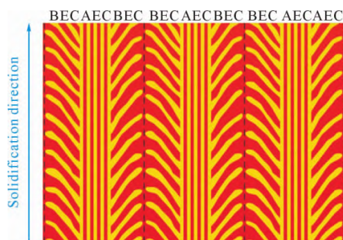
图3 定向凝固 \text{Al}_{19}\text{Fe}_{20}\text{Co}_{20}\text{Ni}_{41} EHEA 中的仿生鱼骨状结构 [18] Fig.3 Biomimetic fish bone-like structure in the directionally solidified \text{Al}_{19}\text{Fe}_{20}\text{Co}_{20}\text{Ni}_{41} EHEA [18]
