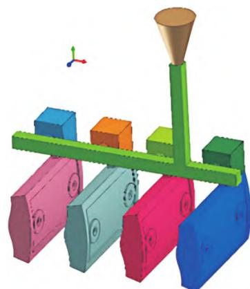
图 8 铸造工艺 C<sup>[37]</sup>Fig.8 Casting process diagram for type C<sup>[37]</sup>
