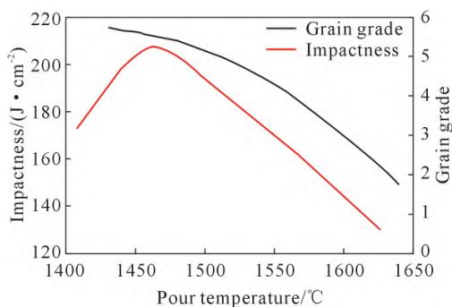
图 10 浇注温度和冲击韧性、晶粒度的关系<sup>[44]</sup>Fig.10 Relationships between pouring temperature and impact and grain grade<sup>[44]</sup>
