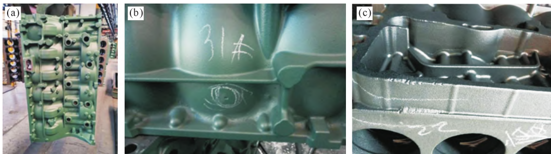
图 2 生产现场铸件缺陷情况:(a) 合格铸件,(b) 铸件气孔缺陷,(c) 铸件砂眼缺陷 Fig.2 Defects in castings at the production site: (a) qualified castings, (b) porosity defect in castings, (c) blister defects in castings
