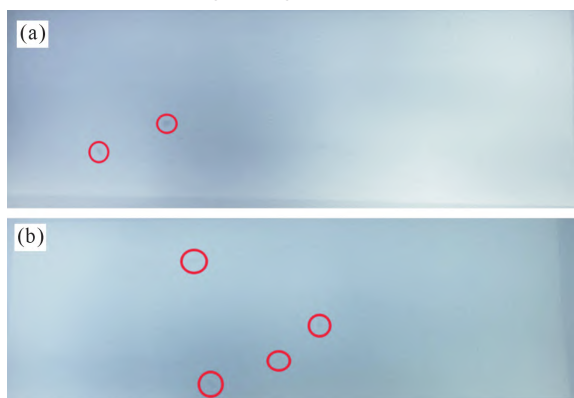
图5 射线检测的夹渣缺陷:(a~b)点状夹渣缺陷 Fig.5 Defect of slag inclusion in RT: (a~b) point slag inclusion
