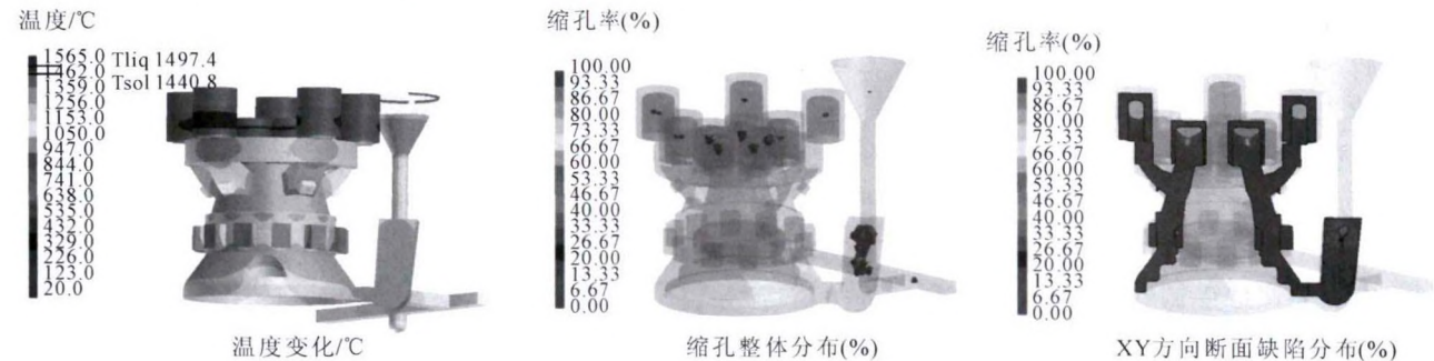
图 6 优化工艺后模拟结果缺陷预测 Fig.6 Defect prediction of simulation results after process optimization
