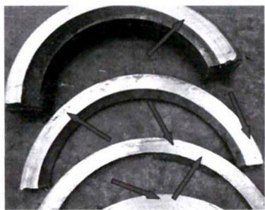
图2 渗油区域断面缩孔缩松分布 Fig.2 Defects distribution of shrinkage cavity and porosity casting in oil-leakage area
