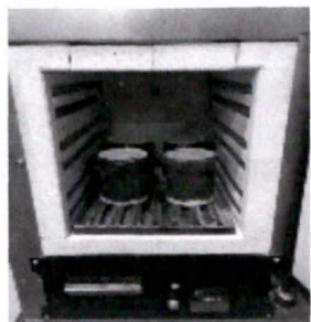
图7 石膏型焙烧 Fig.7 Plaster mold baking
