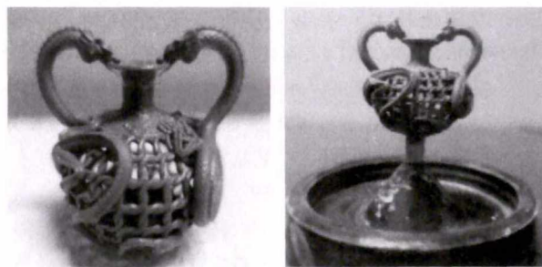
图5 3D 打印的蜡模及装配的蜡树 Fig.5 3D printed wax pattern and assembled wax tree
