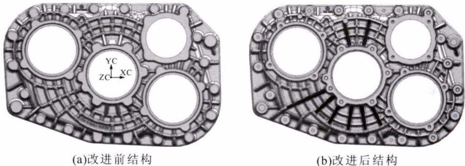
图 7 后盖压铸件改进前后结构对比 Fig.7 Comparison of structure before and after improvement of rear cover die casting
