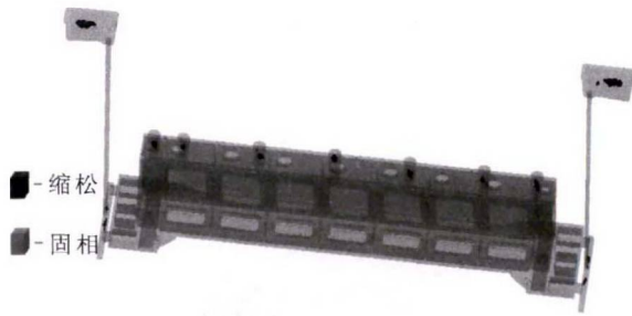
图 7 优化方案铸件缺陷分布 Fig.7 Optimization scheme of casting defect distribution
