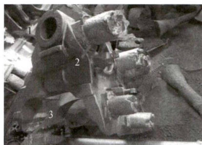
图4 EMB 直浇浇注后产品 Fig.4 casting made by EPC with new evaporative material EMB and direct pouring without burning off evaporative pattern
