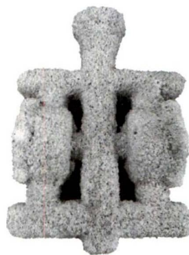
图11 改进方案的模壳 Fig.11 Ceramic shell of improved gating system
