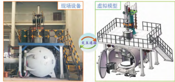
图2 150 kg真空自耗电极凝壳炉的数字孪生示意图 Fig.2 Digital twin diagram of the 150 kg vacuum consumption electrode condenser furnace
