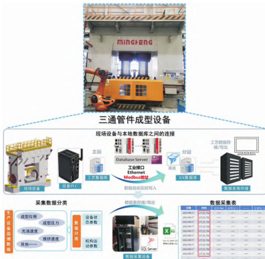
图 6 三通管件成型设备的数字孪生及其工艺数据自动采集与管理 Fig.6 Digital twin of the fabrication equipment for three-way pipes together with its automatic data collection and management
