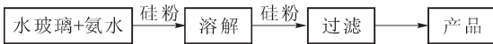
图 1 单质硅溶解法制作硅溶胶流程 [4] Fig.1 Flow chart of colloidal silica preparation by solubilization of elemental silicon [4]
