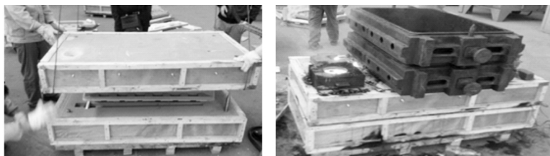
图7 砂芯装配 Fig.7 Sand core assembly
